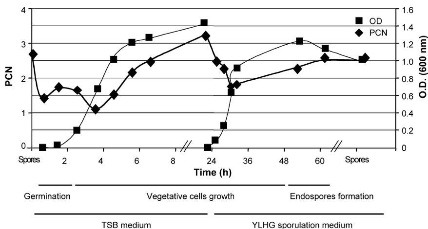
**Fig. 4.** pMTL500Eres PCN variations over the life cycle of *B. cereus*. Spores were incubated in TSB to induce germination and growth and further inoculated in YLHG medium to induce sporulation. The cellular state was monitored by microscopy.
